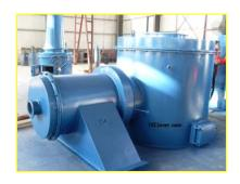
Secondary Chamber & Mix-Combustion Chamber. Residency time 2.0 sec. in post combustion chamber. Virtually
